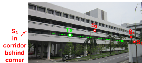
Fig. 7. Picture of the measurement site. The two NLOS nodes are placed on a different floor than the transmitter and the LOS node. The node S_3 is around a corner of the corridor in which the transmitter is placed.
